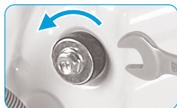
Loosen the 4 transport bolts with a spanner.
