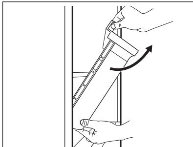
3. Lift and turn the drawer to pull it out of the appliance.
