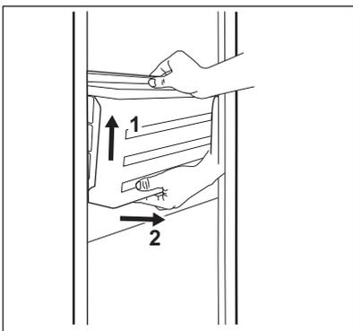
4. Push the rails inside the cabinet to avoid damage to the appliance when closing the door.
