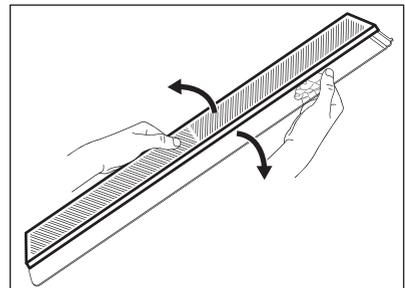
3. Assemble a new membrane into the cover by pressing the edge of the membrane into the cover.
