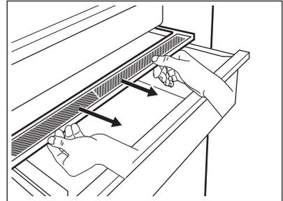
2. If you need to replace the device's white membrane, grab the device in the middle and separate the membrane from the cover by pulling the cover.
