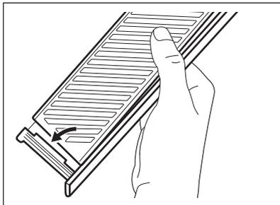
4. Reassemble the humidity control back on the drawer.
