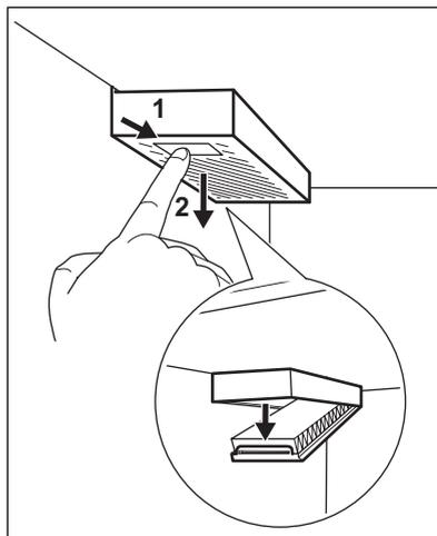
2. Pull out the used air filter.
