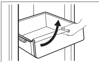
3. Pull the drawer out while lifting it up and detach it from the rails.
