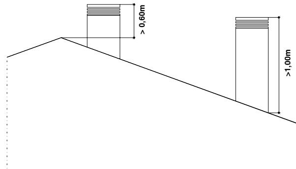
It must be planned accessibility for the chimney maintenance, so its attachment should not be permanent.
