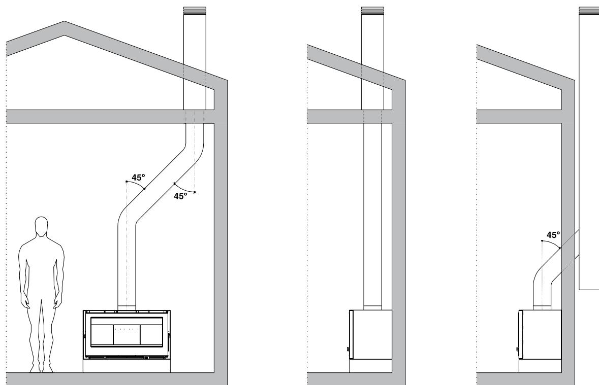
The top of the chimney should be at least at 0,6 metres from the ridge of the roof, otherwise it should be 0,6 metres higher than the ridge. It should be 1 metre above the roof elsewhere. The chimney should be easily accessible for maintenance purposes.
