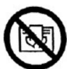
**WARNING:** The meaning of this figure is "*Do not cover*". In order to avoid overheating, do not cover the heater.
