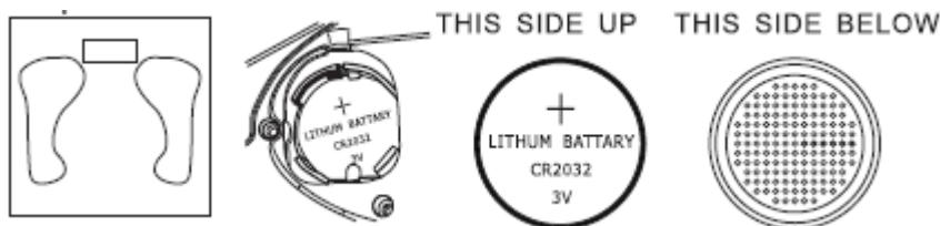
(Note: to insert the battery correctly, the positive pole should be upside, and the negative pole should be downside). After insert the battery, there would be "HI" showing, please do not step on the scale this time. Otherwise, the weighing result would be affected.
