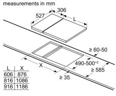
When installing a Domino unit right next to a hob, an assembly kit (HEZ394301) is required.
